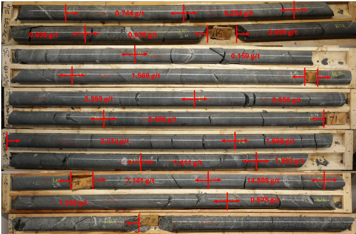
Figure 5. Core photographs indicating sample intervals with Au g/t assays for drill hole RC26-003 (63-77m).
